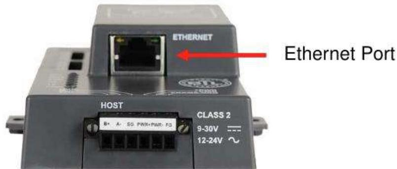
**Figure 8-1: ProtoNode Ethernet Port**
