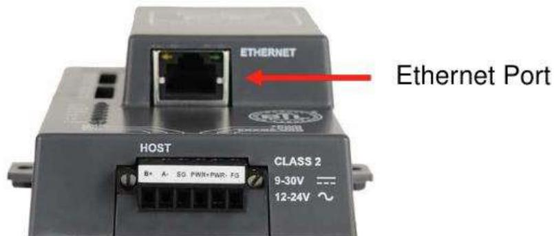
**Figure 4-1: ProtoNode Ethernet Port**
