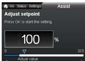
Figure 16: Press "Ok" to select Setpoint.
