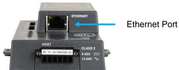
Figure 9: Ethernet port location on the ProtoNode
