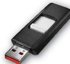
**USB Data Sharing** – Make room on the tool belt for a flash drive as the USB data sharing port has become another important device for commissioning (uploading/downloading settings from one boiler to the next), servicing (downloading data and emailing file(s) to factory for assistance) and analyzing boiler operation (historical info can be downloaded & saved in .CRV formatted files).
